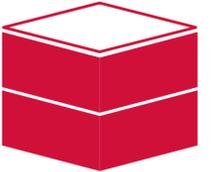
A systemised approach based on volumetric construction involving the production of three-dimensional units in controlled factory conditions prior to final installation. Volumetric units can be brought to final site in a variety of forms ranging from a basic structure only to one with all internal and external finishes and services installed, all ready for installation.
