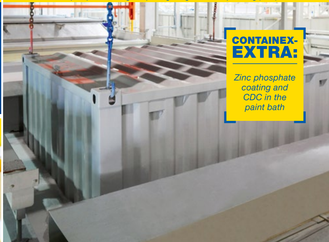
Zinc phosphate coating and priming using cathodic dip coating (CDC)
