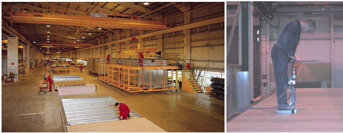
Figure 3.1 Aspects of factory production: (left) an overhead crane and other equipment for handling large panels for the floor, walls and roof; (right) an automatic screw applicator for securing the flooring.
