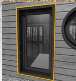
Peripheral sealing of doors, windows and joinery
